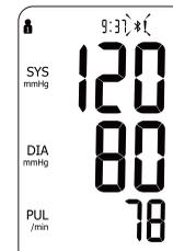
2. This device will proceed to data transmission after measurement. The Bluetooth symbol blinks on the LCD indicates data is transmitting.
